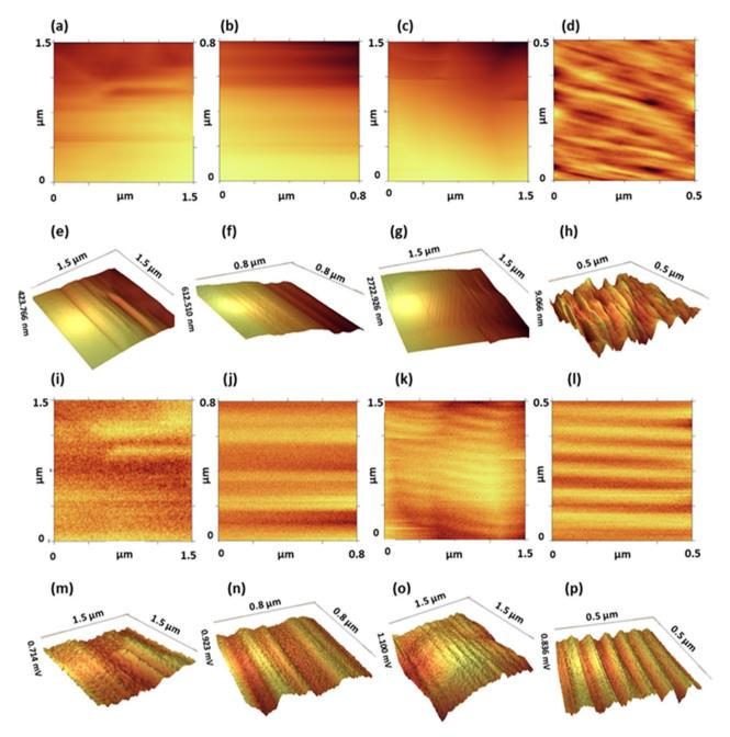
**Figure 3.** MFM images of all samples in Oven-, Autoclave-, Heater-, and LFE-method (left-right). (**a-d**) 2D topography images. (**e-h**) 3D topography images. (**i-l**) 2D amplitude images. (**m-p**) 3D amplitude images of FGPs in Oven-, Autoclave-, Heater-, and LFE-method, respectively (left-right).
