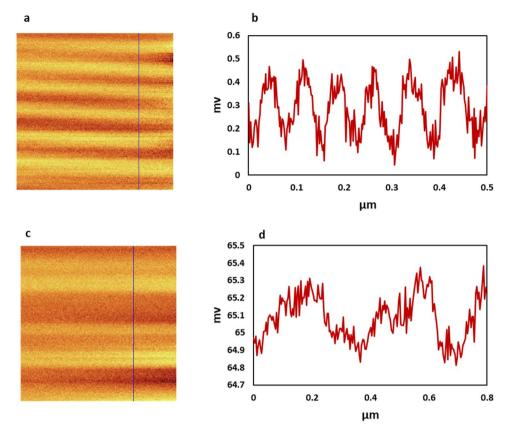
**Figure 4.** Magnetic domains of LFE- and Autoclave-samples and their domain size. Amplitude images and profile of blue line (**a**,**b**) LFE-method. (**c**,**d**) Autoclave-method.
