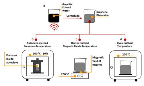
**Figure 1.** Dispersion of graphene and three different methods for investigating the effect of temperature, pressure, and magnetic field on the magnetization of graphene. (a) Dispersion of graphene dispersion by the liquid-phase exfoliation method. (b) Appling temperature and pressure by the Autoclave-method. (c) Appling magnetic field and temperature by the Heater-method. (d) Appling temperature by the Oven-method.
